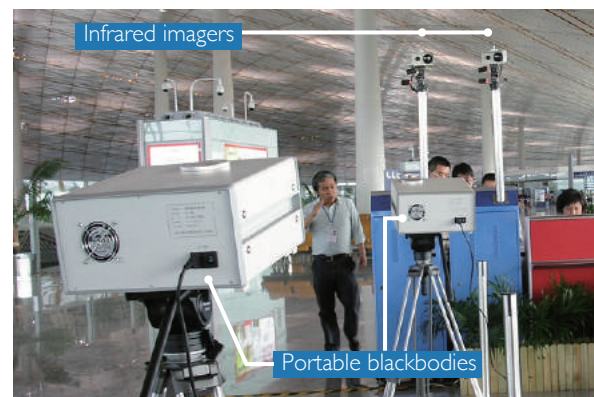
Fig. 6 Use of PBCIRTs for on-site calibration of thermal imagers for fever screening
