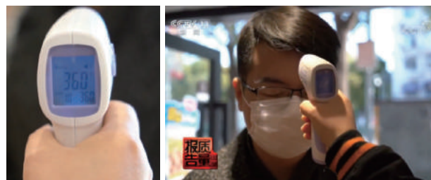
Fig. 2 An infrared forehead thermometer with its application
