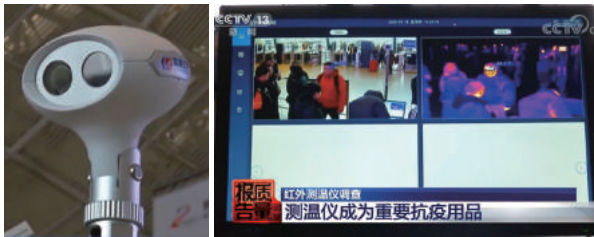
Fig. 3 A thermal imager for fever screening with its application
