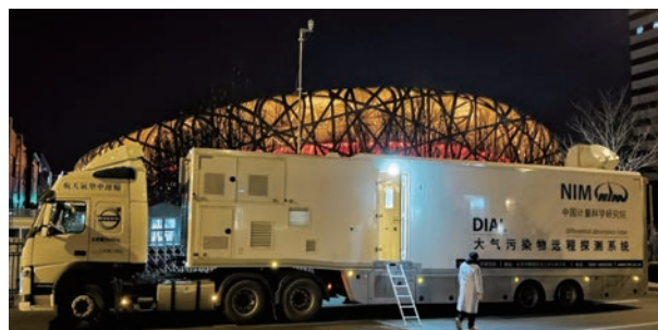
Fig. 12 DIAL in operation at China's National Stadium for air quality monitoring
